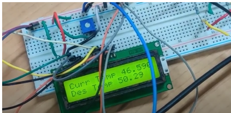
Figure 11: Setting the temperature at 50^{\circ}\text{C}
